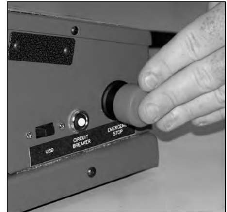
Press in on Emergency Stop Switch to activate emergency stop.
