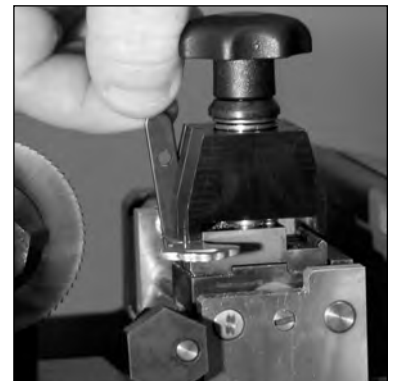
Positioning tip of Calibration Key against Key Stop Tool 1
