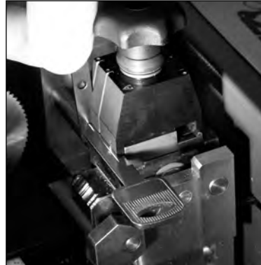
Using Key Stop Tool to position "shoulderless" Key
