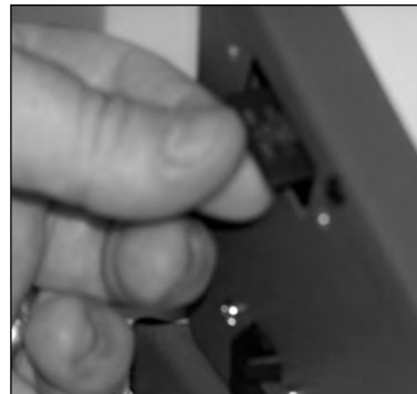
Inserting new SD Card
