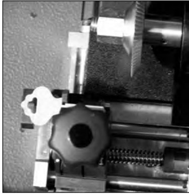
Positioning Calibration Key against Key Gage
